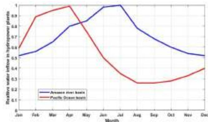
Fig. 13. Monthly water flow variation in hydropower plants located in the Amazonian River and the Pacific Ocean basins in Ecuador. The lines show mean values from 1964 to 2016. Adapted from Ref. [60].
