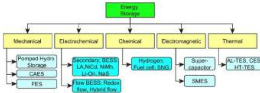
Fig. 1. Classification of energy storage systems based on the form of energy stored. Adapted from Ref. [6].
