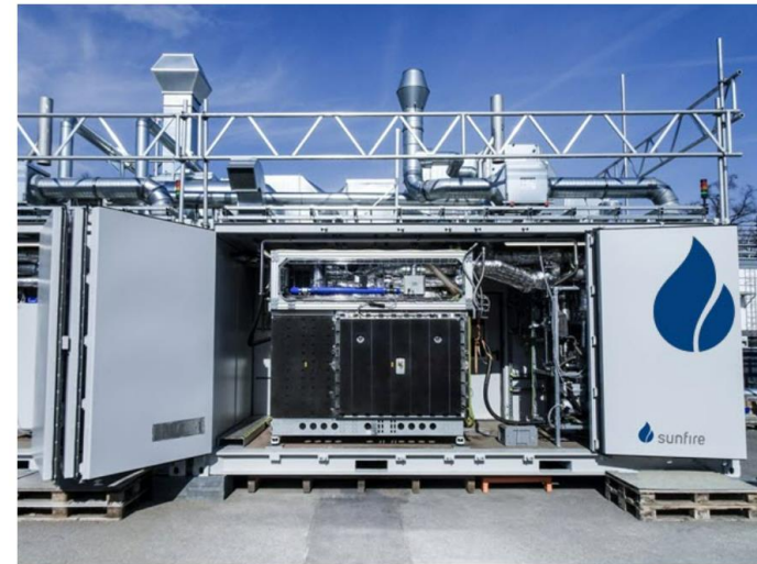
High-Temperature Electrolyser (HTE) Salzgitter Flachstahl GmbH. SOEC 720 kW 200 Nm 3 o 18 kg H 2 /h GrInHy2.0 project Electrical efficiency 84 % (LHV)-2022
